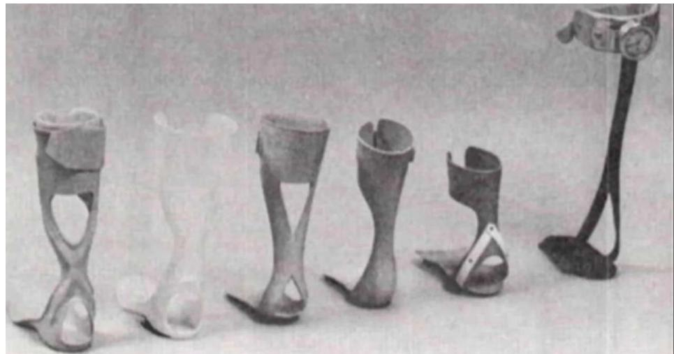
Fig.10 The TIRR Polypropylene Orthoses(Engen 1972<sup>14</sup>)
