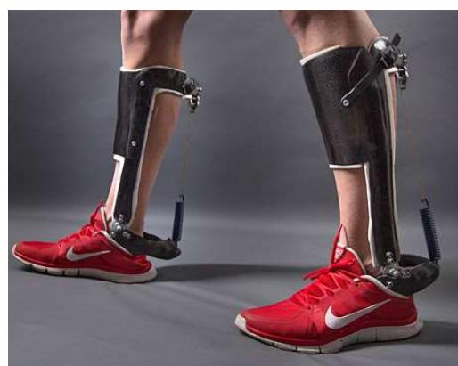
Fig.16 Unpowered exoskeleton Collinsら(2015)<sup>22</sup>
