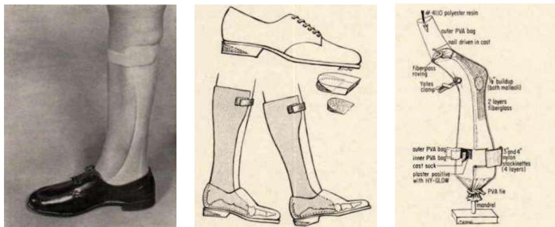
Fig.9 Plastic short leg brace fabrication(Bernard 1967<sup>13</sup>)
