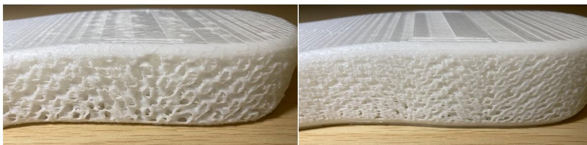
[Fig.5-5-3] Cura Gyroid Infill 12% (左) と Infill 20% (右)
