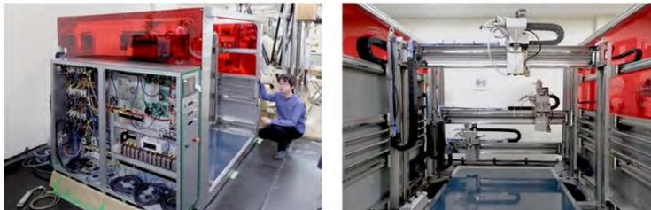
This is a large custom 3D printer that can output objects as large as one cubic meter at a time. By moving three heads at the same time, speedy production can be realized.
