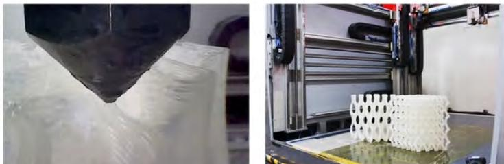
The photo on the left was taken with a tracking camera attached to the nozzle. It makes use of the traces of large pitch lamination to create a surface with a unique expression.
