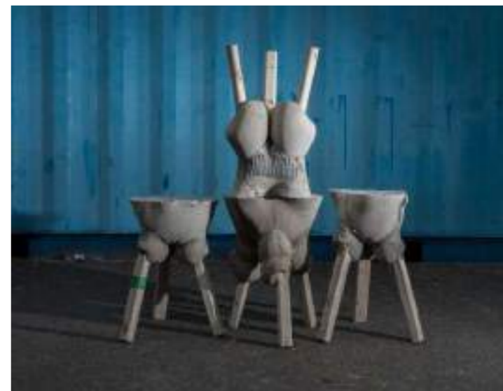
図4：Fabric Formwork Concrete Casting, made by Greig City Academy
