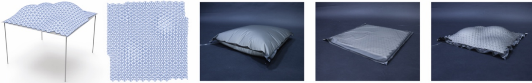
Figure 12: Pneumatic Auxetics provides a morphing sunshade. The amount of sunlight blockage is controlled by three different state changes: air released, inflated with air and deflated.
