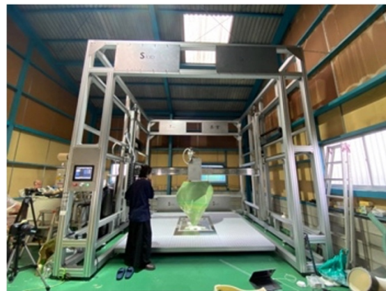
Figure 13: The 1/1 scale pneumatically actuated shell (left). Archi Fab "Chashitsu" is a large FGF 3D printer, with a build area covering 2.8m*2.8m*2.8m (right).
