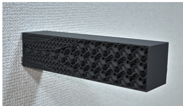
Fig.4. An actual 3D-printed cantilever beam
