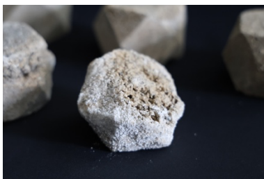
Fig.6 Sample① with pronounced efflorescence
