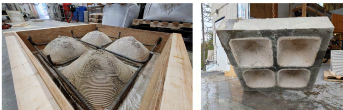
図 18: Parametric waffle slabs: Optimal geometry materialized with additive construction ( https://www.researchgate.net/figure/Fabrication-of-flat-concrete-slab-element-with-mass-customized-formwork_fig5_364152892 より引用)
